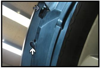
In the wheel well, remove the pushpin (white) and the Phillips head screw (gray). Do this to both sides of the vehicle.
