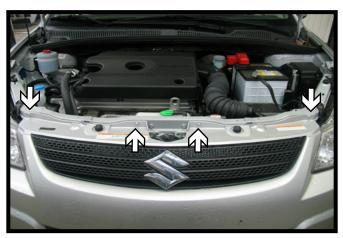
Along the top edge of the fascia, remove the four (4) bolts with a 10MM socket or a Phillips screw driver.
