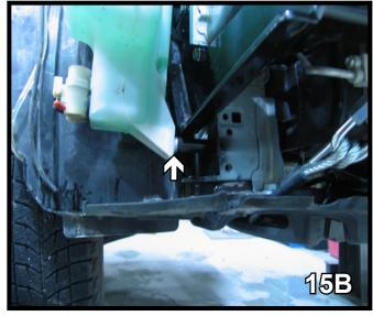
15. Reinstall the washer reservoir using 6MM -1.0 x 30MM hex bolts, 1/4" flat washers and 1 1/2" pipes in the two top holes (15A). In the bottom hole, use a 6MM-1MM X 80MM hex bolt, 1/4" flat washer and 2 1/2" tube (15B).
