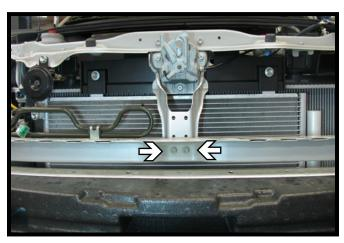
11. Using a 10MM socket, remove two (2) bolts from the center of the bumper. Carefully remove bumper and set aside.
