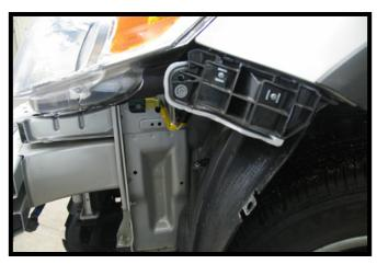
4. To remove fascia, pull it out to the side and forward a little bit. Once fascia is forward there are two clips on top to be removed by pushing in on the fascia and lifting up on the clips to get them over the stops. Set fascia aside.
