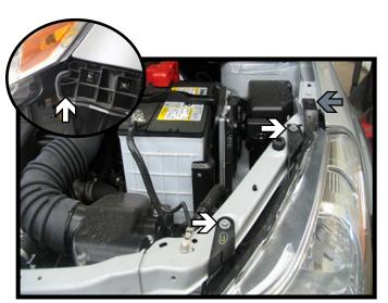
6. Using a 10MM socket, remove two (2) bolts on top and one metric bolt on the bottom of the headlight assembly (white). There is also a pushpin on top that needs to be removed (gray). Pull the headlight assembly forward to remove and disconnect the electrical connections. Do this to both sides of the vehicle.
