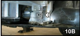
10. Using a marker, make a horizontal line just below the metal bumper. Then with a reciprocating saw, cut into the edge of the frame well and follow it down to the bottom and out. It's very important to follow the frame well because it offsets down at the top. You will then be able to remove that whole portion of the frame well webbing. Do this to both sides of the vehicle.
