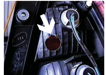
Location for the BX8869 on driver's side.
