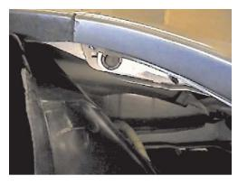
**3.** Just forward of front tire and inside wheel well is one push pin to remove from fascia's upper corner.
