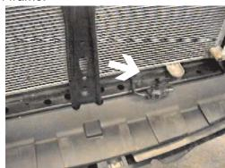
**16.** Bend temperature bracket and sensor back toward radiator. It may be necessary to bend backet more when baseplate is installed and may differ from vehicle to vehicle.
