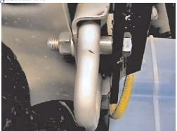
18. Using the baseplate as a template, drill lower hole into lower frame webbing just inside tie down opening. Insert the 3/8" hex bolt into drilled hole and tighten 3/8" lock washer and 3/8" hex nut, both sides. Be sure and use loctite red on all bolts before tightening. Torque all bolts according to torque chart in General Instructions.
