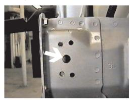
**15.** Using the 17/32" drill bit, drill out the existing larger hole in frame rail, both sides.
