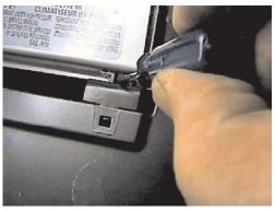
2. Using a small flat screw driver, push the four tabs down between the top edge of fascia and upper cross member while pulling fascia forward to release from cross member.
