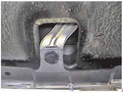
**6.** Remove push pin from tab on lower center edge of fascia.
