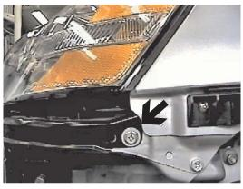
**8.** Remove metric bolt from lower side of head light assembly using the 10MM socket, both sides.
