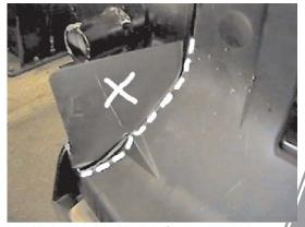
12. Using the utility knife mark and cut lower air dam from both sides. This will allow open area for baseplate installation.
