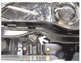
**9.** Remove metric bolt from front of head light assembly with the 10MM socket, both sides.
