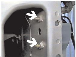
14. Using the flat chiesel, remove the two weld nuts inside frame rail, both sides. This will allow enough room for nut plate on the inside of frame.
