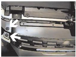
1. Remove metric bolt with the 10MM socket and one phillips push pin on top edge of grill, both sides.
