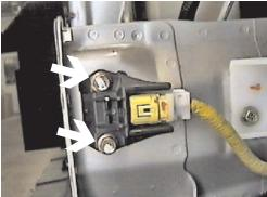
**13.** Using the 10MM socket, remove two metric bolts from air bag sensor and carefully set out of the way, both sides.
