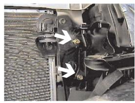
**10.** Remove two metric bolts from headlight assembly next to radiator, both sides, pull assemblies forward, unplug and set aside.
