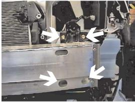
**11.** Remove four metric bolts from both sides of metal bumper, pull forward and set aside.
