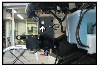
16. Slide the baseplate onto the vehicle lining up the existing hole in the frame with the baseplate (white). Install a 1/2"-13 x 1-1/4" bolt into the hole with 1/2" flat washer, lock washer and nut on the inside of the frame. Do this on both sides of the vehicle. Level the baseplate and fully tighten the 1/2" hardware. Using a 13/32" drill bit, drill the remaining six (6) holes of the baseplate thru the frame (gray). There are three (3) on each side.
