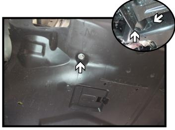
12. **2014 Models:** Drop the front of belly pan down for baseplate installation. Using a 12MM socket, remove the two (2) screws from the underneath. Then remove the two (2) push pins from the sides (inset). Unsnap the front lip from the brackets.
