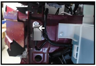
2012-13 Models: Using a 10MM socket, remove the screw from the sensor on the driver side.
