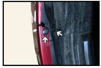
Remove the two (2) push pins from the outer edge of the wheel well. Do this on both sides of the vehicle.
