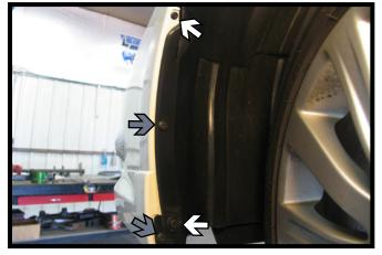
Remove the two (2) push pins from the outer edge of the wheel well (white). Then using a Phillips screwdriver, remove the two (2) screws (gray). Do this on both sides of the vehicle.
