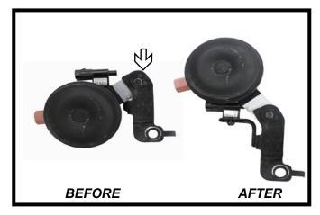
11. Using a 10MM socket, loosen the bolt on the backside of the bracket. Position the arm as shown and retighten the bolt. Reinstall the horn bracket to the vehicle and hook up the electrical connections.
