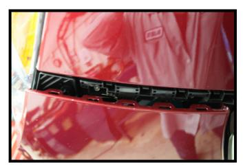
Unsnap the corners of the fascia from the fender. Remove the fascia from the vehicle, disconnecting any electrical connections and set the fascia aside.
