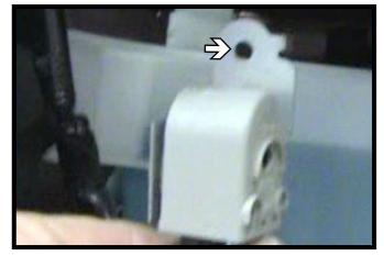
Using a 13/32" drill bit, ream out the existing hole in the sensor bracket on the driver side.
