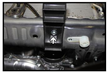
13. **2014 Models:** Using a 10MM socket, remove the screw from the belly pan bracket and set aside. Do this on both sides of the vehicle.
