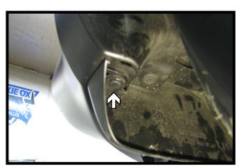
Underneath in front of the tire, use a flat screwdriver to remove the push pin in the corner. Do this to both sides of the vehicle.
