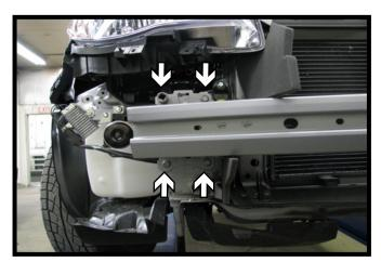
7. Remove the metal bumper, using a 12MM socket, remove the four (4) bolts from the bumper. Do this on both sides of the vehicle.
