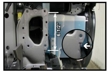
8. Using a reciprocating saw, make a notch down 6-1/2" from the top of the frame and flush with the lower outer flange of the frame. Do this on both sides of the vehicle.
