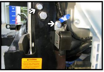
14. Install 3/8"-16 x 1-1/4" bolts, 3/8" flat & lock washers and 3/8" lock nuts into the top holes of the baseplate. Do this on both sides of the vehicle.
