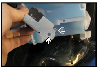
13. On the driver side, using a 13/32" drill bit, ream out the hole in the sensor bracket (white). Next flatten or trim off the alignment tab (gray).
