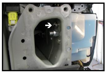
12. After drilling out the holes, use a flat chisel and knock off the nut on inside of the frame.
