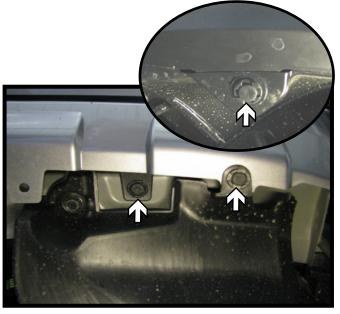
4. Using a flat screwdriver, remove six (6) push pins from the underside of the fascia. There is one (1) in front of the tire and two (2) in the towards the middle. Do this on both sides of the vehicle. Pull fascia corners outwards, then pull fascia forward to remove.
