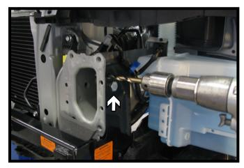
11. Tip the baseplate into position. Install 1/2"-13 x 1-1/4" bolts, 1/2" flat & lock washers and 1/2" lock nuts into the existing frame holes. Level the baseplate and tighten down the bolts.
