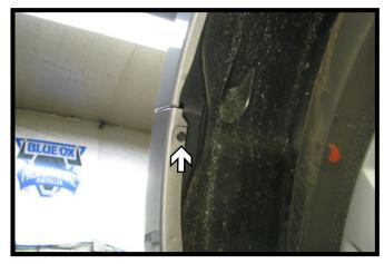
2. Just forward the front tire, push the pin in the center to release. Do this to both sides of the vehicle.
