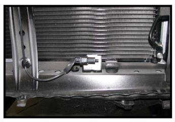
9. Bend the temperature sensor backwards at an angle towards the radiator.
