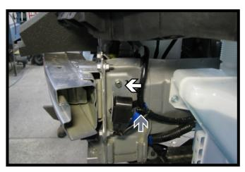
On the driver side, using a 10MM socket, remove the bolt above the sensor (white). Unplug the wiring (gray arrow).
