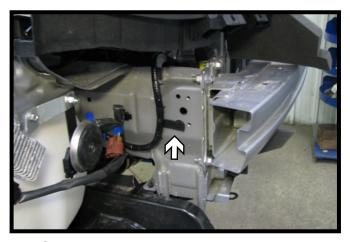
6. On the passenger side, remove the wiring push pin.
