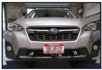
25. Hold the fascia as close to its original position, mark and trim the fascia around the convenience links and attachment tabs. Reinstall the fascia and fascia cover.
