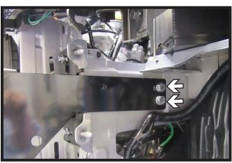
20. Remove the two (2) bolts on the side of the baseplate, one at a time. Apply Loctite® Red and tighten to appropriate torque. Do this on both sides of the vehicle.
