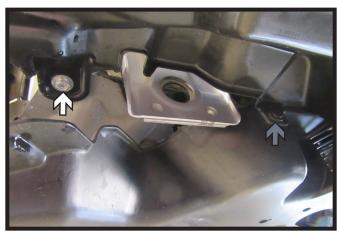
7. Pull down the belly pan and using a 10MM socket remove the one (1) bolt (white) as indicated. Then remove the one (1) push pin (gray). Do this on both sides of the vehicle.
