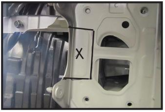
17. Using a reciprocating saw remove the indicated off set area so that it is flush with the frame.
