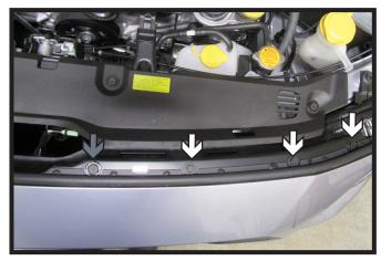
1. Using a 10MM socket, remove the four (4) bolts (white) from the top edge of the fascia. Then remove the two (2) push pins (gray).
