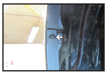
Remove the one (1) push pin from inside of the wheel well by pressing on the center. Do this on both sides of the vehicle.
