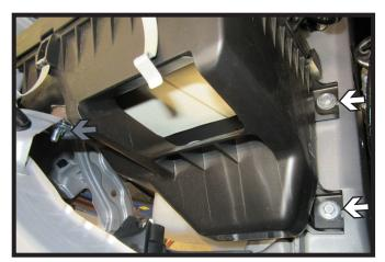
12. Using a 10MM socket remove the two
