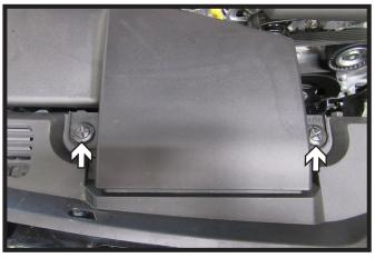
10. Using a flat head screw driver turn top two (2) screws 1/4 of a turn and remove plastic piece from the passenger side of the vehicle, to be reinstalled later.
