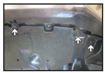
3. Remove five (5) push pins from the underside of the fascia. Do this on both sides of the vehicle.
