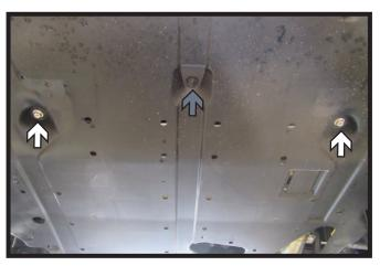
15. Using a 12MM socket remove the two (2) bolts (white) from the belly pan of the vehicle. Then remove the one (1) push pin (gray). The belly pan will hang loose once these are removed.
