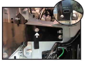
21. Start one (1) 3/8" bolt with lock washer and insert 3/8" nut plate with 14" wire through access hole on the bottom side of the baseplate (inset) and attach to back side of bolt. Then place flat spacer plate between baseplate and frame. Do this on both sides of the vehicle.
