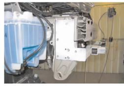
12. Slide baseplate onto tie down bracket and up to align with existing holes for air bag sensors, both sides. Using the existing metric bolts for sensors, tighten metric bolts with the 10MM socket both sides. Be sure baseplate is level with vehicle. NOTE: Baseplate is painted white to increase visiblity in photo.
