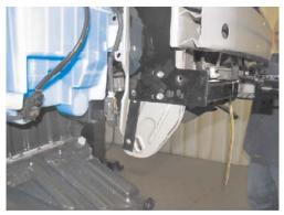
**15.** Insert spacer plate between tie down bracket and baseplate to align with the two holes on the back edge of baseplate end, both sides.
