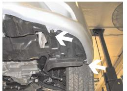
**5.** Remove the two metric bolts just forward of the front tire, on the bottom side of fascia, using the 10MM socket, both sides.
