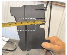
**11.** Measure and mark from the back edge of air dam forward 1 1/2" on both sides and cut out area with the utility knife, both sides.
