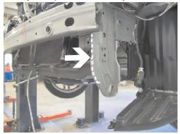
**9.** Using the reciprocating saw, cut and remove front webbing of tie down bracket, both sides. This will open area to allow baseplate to slide onto the outside of tie down bracket and frame.
