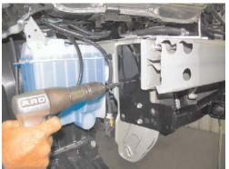
**13.** Using the baseplate as a template, drill the holes into the frame and webbing with the 13/32" drill bit, both sides. **Do not drill the two back holes for the sensors.**
