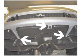
6. Remove three metric bolts from lower edge of fascia tabs with the 10MM socket. Pull fascia forward, set aside and remove styrofoam from metal bumper.
