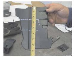
10. Remove push pin from air dam and pull forward to release, both sides. Measure 2 1/4" and 4 3/8" down from the top of air dam, both sides.
