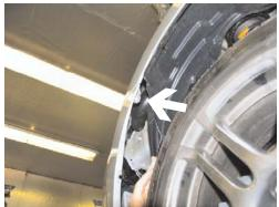
**4.** Forward of front tires inside wheel well on fascia's upper corner is one metric bolts to remove with the 10MM socket, both sides.
