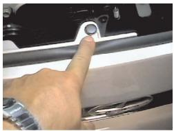
**2.** Remove push pin from top edge of fascia just forward of hood latch.
