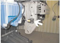
**7.** Using the 10MM socket, remove two metric bolts from air bag sensor, both sides and carefully tie up out of the way.
