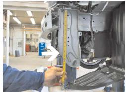
**8.** Measure 10 1/2" down from the bottom side of upper frame webbing and mark the front webbing on tie down bracket.
