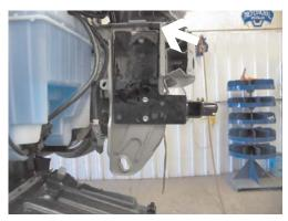
14. Insert the 3/8" nut plate into opening on top edge of frame just behind bumper bracket and align with top drilled hole. Tighten 3/8" hex bolt and lock washer, both sides. Be sure to use loctite red on all bolts before tightening. Tighten all bolts according to Torque Chart in General Instruction Sheet.
