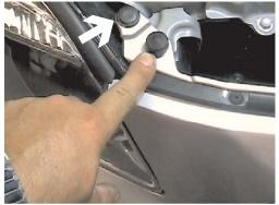
1. Remove push pin from top edge of fascia just inside of head light assembly (white arrow), both sides. Lift top portion of hood bumper pad up to release, pull lower body up out of fascia and set aside, both sides.
