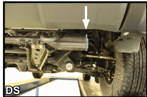
3. Locate the frame extension, with a reciprocating saw remove the end portion of the cross member slightly so it is flush with the tab. Be sure to paint edges with a high quality paint in order to prevent rusting.
