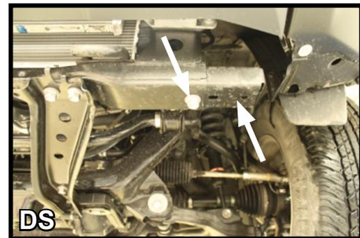
2. On 2011-2012 models only, locate the frame extension, remove the bolt using a 12MM socket and slide outer tube out. The outer tubes will not be reinstalled.
