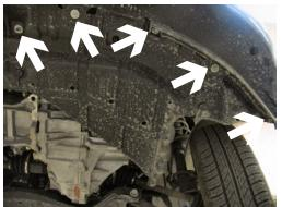
**3.** Remove the nine metric bolts from the lower edge of fascia with the 10MM socket (Driver's side shown).
