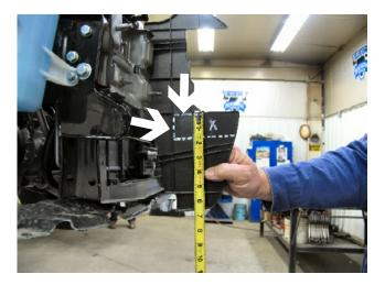
7. Release the two clips on the back side of radiator support and pull air dam forward set aside, on both sides (Left photo above). Measure down 1 7/8" and mark the air dam from the edge just below where the metal bumper would set. Cut and remove the area below metal bumper back to first rib, down to 1 7/8" mark and cut a line forward to front edge. This will open area for baseplate.
