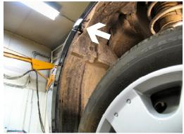
2. Just forward of front tire is one metric bolt to remove with the 10MM socket, on both sides.
