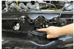
1. Remove the push pin from just below hood latch on top side of fascia.
