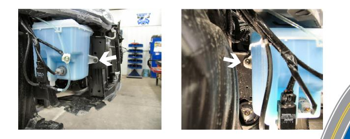
**8.** Using the 10MM socket, remove the front metric bolt from windsheild washer reservoir (Left Photo). Loosen the metric bolt on the back side of reservoir (Right Photo).
