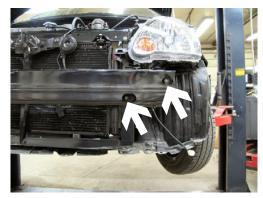
5. Remove the two metric bolts from metal bumper using the 12MM socket, both sides. Pull metal bumper forward and set aside.
