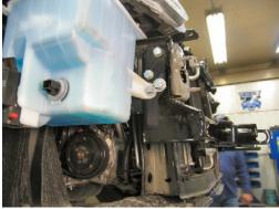
**10.** Insert nut plates into opening on the end of frame rail to align with drilled holes on the passenger's side, tighten the three 3/8-16 hex bolts lock washers and flat washer, please refer to page 5. **Be sure and use Loctite on all bolts before tightening. Torque all bolts according to torque chart in General Instructions.**
