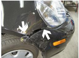
4. Using the small flat screw driver, release the clip just outside headlight assembly on seam between the fender and front fascia, both sides. Pull corner of fascia down and to the side of vehicle, pull fasica forward and set aside.
