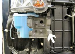
6. Remove the two metric bolts from bumper bracket, pull forward and set aside, on both sides.
