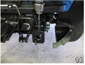
14. With the baseplate on top of the frame rail extension, use the baseplate as a template to drill two holes in the top of the extension with the 13/32" drill bit. Insert 3/8" nut plates into frame rail extension and align with drilled holes. Install 3/8-16 x 1 1/4" bolts and 3/8" lock washers to the baseplate and tighten to nut plates using the 9/16" socket. Trim nut plate wires. Do this to both sides of the vehicle.
