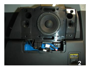
Use a flat screwdriver to pry upward on the panel below subwoofer to remove it. Or, pull forward on upper part of panel. Photo shows panel removed.
