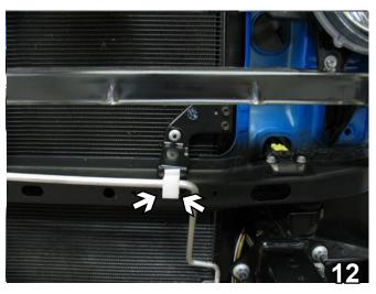
12. On the driver's side, squeeze the back side of the plastic retainer clip holding the coolant tubing. Pull retainer clip forward to release the coolant tubing from the bracket.
