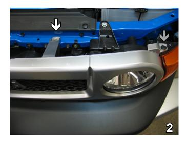
Using a 10mm socket or Phillips screwdriver, remove the hex bolt from the grille support bracket (see white arrow). Remove the pushpin from the upper, outside edge of grille assembly (see grey arrow). Do this to both sides of the vehicle. Set bolts and pushpins aside to be reinstalled later.
