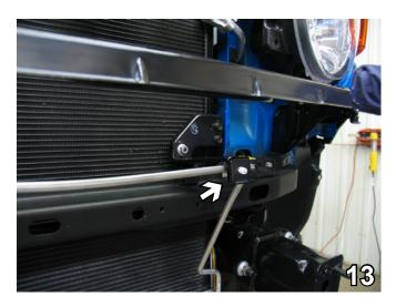
13. Slide the coolant tube behind the bracket. Rotate the retainer clip and insert into the back side of original bracket location to open the area for baseplate installation.
