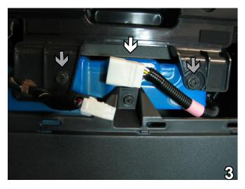
Disconnect the electrical connection (see white arrow). Remove two Phillips screws (see grey arrows). Set screws aside to be reinstalled later.
