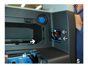
5. Using a flat screwdriver, pry off the taillight panel. In the subwoofer recess, (see white arrow) angle a 10mm deep socket upward to reach two metric bolts in taillight area (see grey arrows). Use a 10mm wrench on the other side of the metric bolts to remove them. Set all aside to be reinstalled later.
