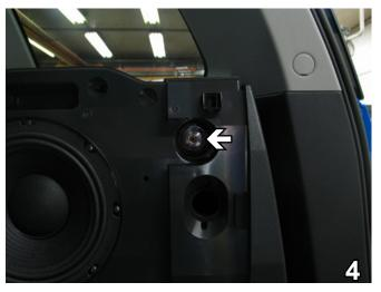
Remove one Phillips screw from each of the upper corners of the subwoofer case. Remove the subwoofer. Set screws and subwoofer aside to be reinstalled later.
