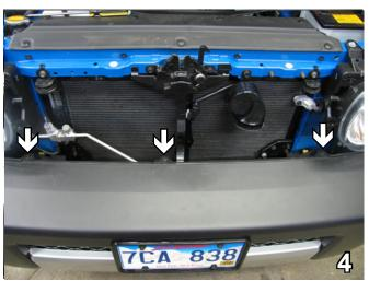
Remove three pushpins just behind the top edge of the bumper. Set pushpins aside to be reinstalled later.
