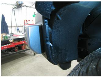
8. Grasp the top edge of the fascia's corner, just forward of the front tire and carefully push the fascia's corner towards the front tire, then pull to the side to release fascia. Do this to both sides of the vehicle. Pull fascia forward to remove. Set fascia aside carefully to be reinstalled later.
