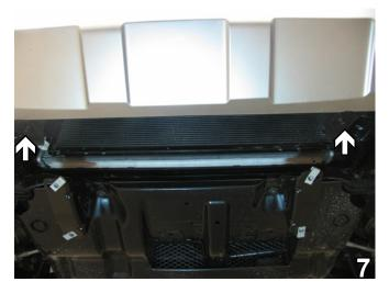
Using the 10mm socket, remove two metric bolts from the bottom edge of the fascia, just forward of the radiator. Set bolts aside to be reinstalled later.
