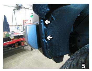
Using the 10mm socket, remove two metric bolts from the outside edge of wheel well, just forward of the front tire. Do this to both sides of the vehicle. Set bolts aside to be reinstalled later.
