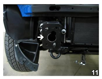
11. Using the 1 1/4" hole saw, drill out the center of the frame rail end plate. *Note: The cut should overlap the existing hole*. Do this to both sides of the vehicle.
