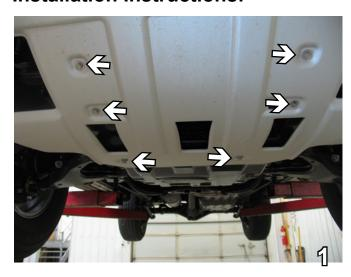
Using the 12mm socket, remove six metric bolts from the belly pan. Set belly pan and bolts aside to be reinstalled later.
