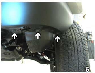
Using the 10mm socket, remove three metric bolts from the bottom corner of fascia, just forward of the front tire. Do this to both sides of the vehicle. Set bolts aside to be reinstalled later.
