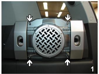
Use a 3/16" Allen wrench to remove four screws from the sub-woofer panel in the rear cargo area. Pull the panel forward to remove. Set panel aside to be reinstalled later.
