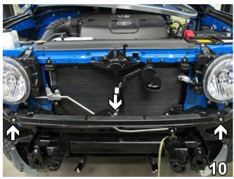
10. Using the 10mm socket, remove three bolts from the fascia support crossbar. Pull the crossbar forward to remove. Set bolts and crossbar aside to be reinstalled later.
