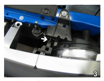
3. Just forward of the radiator, on the outside edge of the headlight assembly, press the tab in (see white arrow) and pull the grille slightly forward to release the upper clip. Do this to both sides of the vehicle. Pull grille forward to release the three lower grille clips. Set grille aside to be reinstalled later.
