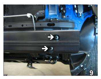
Using the 14mm socket, remove two metric bolts from the metal bumper. Do this to both sides of the vehicle. Pull metal bumper forward to remove. Set bolts and bumper aside to be reinstalled later.
