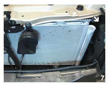
On the side of the radiator, pull the air dam forward to remove. Do this to both sides of the vehicle. Set air dams aside to be reinstalled later.
