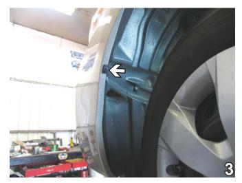
On outside edge of wheel well, turn screw 90 degrees with the flat screwdriver to remove.
