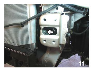
11. Using the flat cold chisel, remove the square nut on the inside of the frame rail. Do this to both sides of the vehicle.
