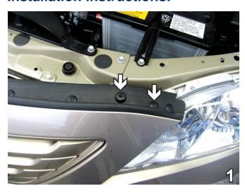
Remove two Phillips pushpins from top of fascia - the second and third in from the headlight. Do this to both sides of the vehicle. Set pushpins aside to be reinstalled later.
