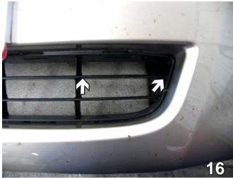
16. Lay the fascia face up on a smooth, flat surface. Using the hack saw blade, remove the top rib in the upper corner of the grille style. Do this to both sides of the vehicle.
