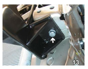
13. Using the baseplate as a template, drill into the bottom of frame with the 13/32" drill bit. Insert nut plate and align to drilled hole. Install 3/8-16 x 1 ½" bolt with 3/8" lock washer and tighten. Do this to both sides of the vehicle.
