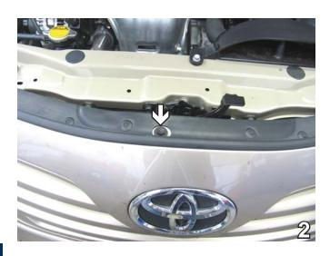
2. On the top center of the fascia, use the 10mm socket to remove one metric bolt. Set bolt aside to be reinstalled later.
