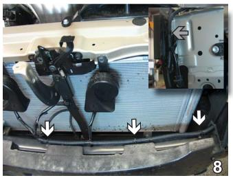
8. On the driver's side, disconnect the horn cable (with fog light connector, if so equipped) from a tie clip on the back of metal bumper (see grey arrow of inset). Disconnect the cable from three tie clips behind metal bumper (see white arrows). On the passenger's side, disconnect the horn cable from a tie clip on the back of metal bumper. Move the cables out of the way to prepare the area for baseplate installation.
