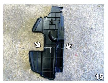
15. Using the utility knife, cut the air dam (ribbed side up) horizontally and slightly below the midpoint of the air dam. Do this to both air dams. Reinstall the upper section of air dams.
