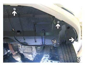
Using the 10mm socket, remove three metric bolts from front edge of belly pan (see white arrows). Do this to both sides of the vehicle. On drivers side, remove one metric bolt from rear corner of belly pan (see grey arrow). Set bolts aside to be reinstalled later.
