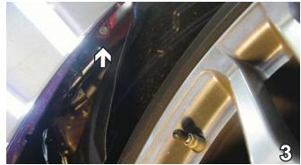
3. Using a 10MM socket, remove one metric bolt from inside front wheel well on fascia's upper corner. Repeat for both sides of vehicle. Set bolts aside to be reinstalled later.
