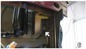
6. Remove one Phillips push pin from air dam. Set aside air baffle for later reinstallation.
