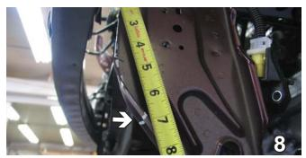
8. Measure 7" down from the bottom side of metal bumper to the lower front tie down bracket webbing, do to both sides.
