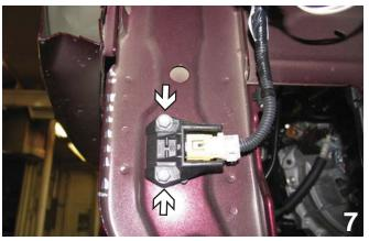
Using a 10MM socket, remove two metric bolts from air bag sensor. Set aside bolts and air bag sensor for later reinstallation.
