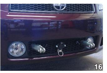
16. Reattach air dam. Align the fascia to its original position and using a side cutters, remove area around attachment tab receiver and quick link to allow it to come through the fascia. Do this to both sides of the vehicle.
