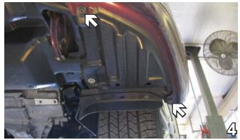
4. Using 10MM socket, remove two metric bolts just forward of the front tire on bottom side of fascia. Do this to both sides of vehicle.
