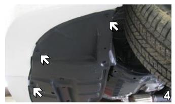
Using 10MM socket, remove seven metric bolts underneath the fascia.
