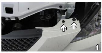
Using a Phillips flat screwdriver, remove one plastic push pin and one metric from both sides. There is also one push pin from the center by the hood latch to remove. Set push pins and bolts aside to be reinstalled later.
