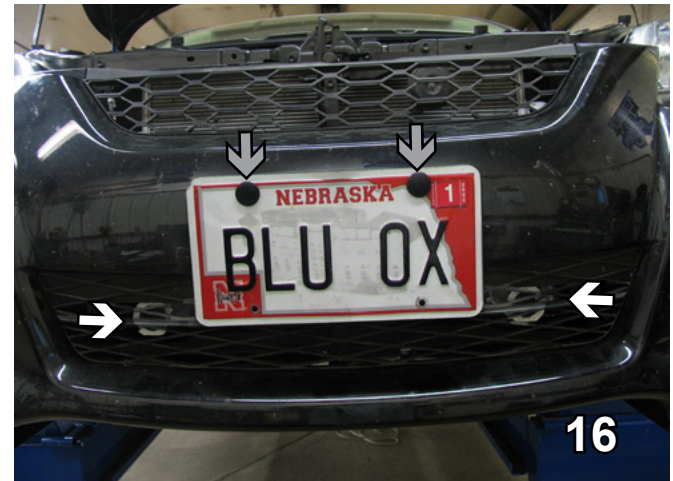
16. Hold the fascia as close to its original position as possible, mark and trim the grill with a utility knife to allow the baseplate receivers to come through (white arrows). Reinstall the fascia. The two license plate screws on the top may have to be raised up about 1/2" (gray arrows).
