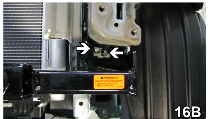
16. Reinstall the frame extension with two bolts on the top and two on the bottom. Do this on both sides.
