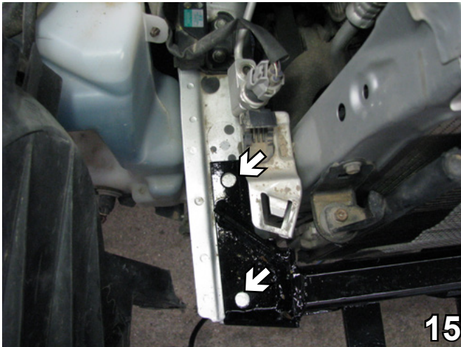
15. On the passenger side, using the baseplate as a template, drill the two holes with the 17/32" drill bit.
