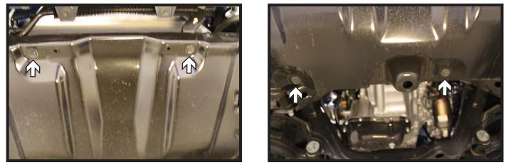
2. Using a 12MM socket, remove the four (4) screws from the belly pan on the underside of the vehicle.
