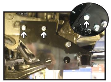
Using a 1/2" drill bit, ream the lower existing hole thru the frame. Install the 1/2" hardware and fully tighten the 1/2" bolt and two (2) existing bolts (inset).
