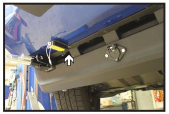
14. **Optional Breakaway:** Install the breakaway in the desired location using one of the existing lower outer valance screws.
