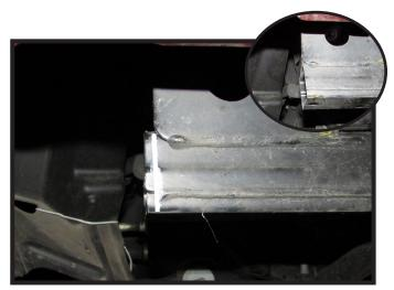
4. Using a reciprocating saw trim the indicated area so that it is flush with the bracket above as shown in inset. Do this on both sides of the vehicle.
