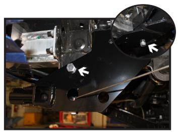
10. Install the spacer tube thru the frame on the driver side. Position the DS baseplate onto the frame and install the 1/2" x 4" bolt and hardware. Do not fully tighten.
