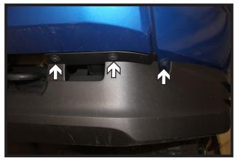
Using a 10MM socket, remove the four (4) screws from the inside edge of the lower valance. There are two (2) on each side (left). Continue along the outside of the valance removing the nine (9) screws along the edge (right). Set the valance aside.
