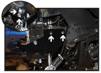
Using a 1/2" drill bit, drill the lower existing holes thru the frame. Install the 1/2" hardware and fully tighten both bolts (inset).
