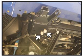
7. Position the PS baseplate onto the vehicle and install the two (2) existing tow hook plate bolts thru the baseplate into the frame. Do not fully tighten.
