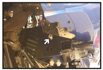
Slide the spacer tube into the frame. Install the 1/2" x 4" bolt thru the outside of frame with the 1/2" hardware on the inside. Do not fully tighten.
