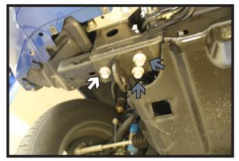
3. Using a 17MM socket, remove the bolts from the frame extensions. There is one (1) on each side (white). Set the extensions aside they will not be reinstalled.
