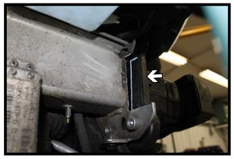
Place the bumper back to the frame. Mark the backside of the bumper around the area trimmed off the frame on both sides. Using a reciprocating saw, trim off the backside of the bumper. Then reinstall it to the vehicle.
