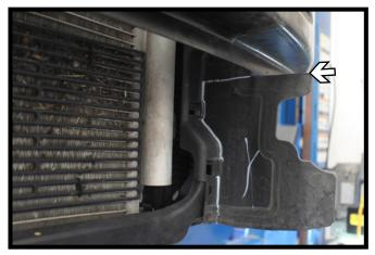
14. Trim the shrouding flush with the bottom of the bumper back the joint then following the joint down to the bottom. Do this on both sides of the vehicle.
