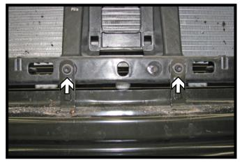
11. Using a T30 Torx, remove the two (2) screws from the center of the bumper. Set the bumper aside.
