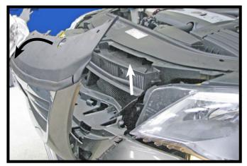
8. Pull the center of the grille forward (black) and lift the inner cover up and out (white). Set the grille aside.
