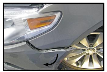
7. Pull the corners of the fascia away from the vehicle and disconnect all electrical connections. Remove the fascia and set aside.
