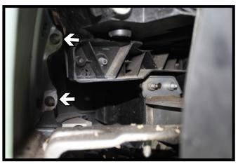
6. **Passet Only:** Using a 10MM socket, remove the four (4) screws from the backside of the fascia behind the wheel wells. There are two (2) on each side.
