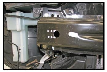
On the passenger side only, using a reciprocating saw, cut two (2) horizontal slits in the bumper as shown. Bend the tab inwards to allow nut plate access.
