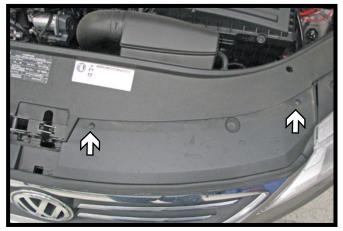
CC: Using a T25 Torx, remove the four (4) screws from the top edge of the fascia. There are two (2) on each side.
