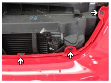
2. Using a 25 Torx, remove the six (6) screws at the top of the fascia. There are three (3) on each side.
