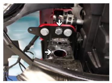
Install a 1/2"-13 x 1-1/2" bolt and 1/2"-13 whiz lock nut in the existing frame hole.
