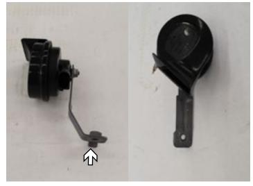
14. Flatten out the horn bracket with a hammer on a solid surface. Then remove the side tab with pliers or vise-grips by twisting back & forth (shown above to left). Bracket should look like right hand picture when done. Repeat on other horn.
