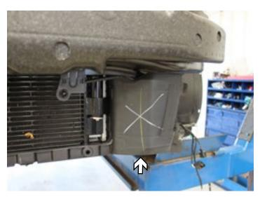
7. After front fascia is removed, locate and remove the two (2) plastic shrouds at the front of vehicle on both sides. These will not be used during re-installation of front fascia.
