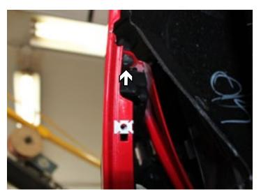
4. Behind the wheel well cover remove the one (1) upper fascia screw with a 25 Torx. Do this to both sides of the vehicle.
