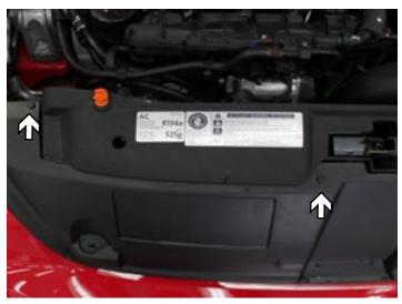
1. Remove the four (4) push pins from the top edge of the radiator cover. There are two (2) on each side. Then remove cover from vehicle.
