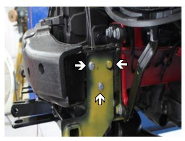
13. Install the three (3) 3/8"-16 x 1-1/4" bolts, 3/8" lock washers and 3/8"-16 nut plates w/wires using the 1-1/4" holes on top of frame to insert nuts. Repeat on other side of vehicle.
