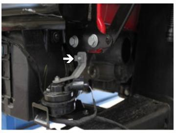
10. Using a 50 Torx, remove the one (1) screw at the top of the horn bracket, unhook the wiring and set aside. Repeat on other side.
