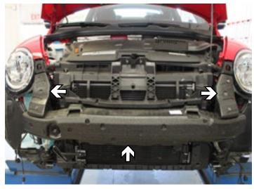
Remove the three (3) foam fascia support pieces. DO NOT discard these will be reinstalled.
