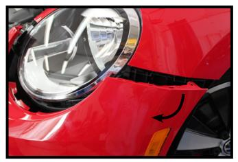
6. When removing front fascia, pull straight out and unhook both the side marker and running light wiring on both sides of vehicle.
