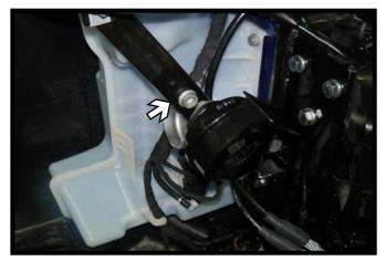
19. To relocate the horn, drill a hole thru the brace and install the horn bracket to the brace. Remove the horn from the bracket and bend the bracket around. Reinstall the horn to the bracket and reconnect the wiring. Do this on both sides of the vehicle.
