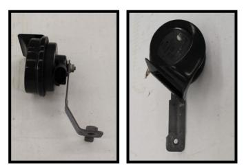
Flatten out the horn bracket with a hammer on a solid surface. Then remove the side tab with pliers or vise-grips by twisting back & forth (shown above to left). Bracket should look like right hand picture when done. Repeat on other horn.
