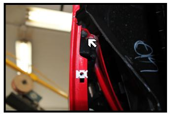
4. Behind the wheel well cover remove the one (1) upper fascia screw with a 25 Torx. Do this to both sides of the vehicle.
