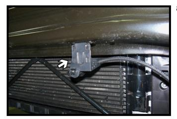
8. Remove the air temperature sensor from the bumper and set aside.
