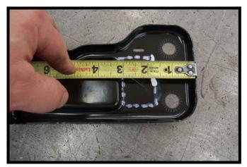
Cut a opening in the brace, approximately 1-1/2" down from the top down to the rib and approximately 3/4" from the sides. Do this on both braces.
