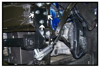
15. Using a 13/32" drill bit, drill the three (3) holes thru the frame. Install 3/8"-16 x 1-1/4" bolts with lock washers into the holes and 3/8"-16 nut plates on the inside of the frame. Do this on both sides of the vehicle. Fully tighten all fasteners.
