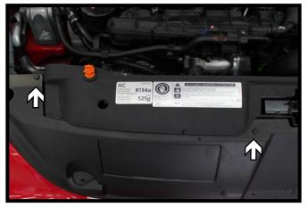
1. Remove the four (4) push pins from the top edge of the radiator cover. There are two (2) on each side. Then remove cover from vehicle.
