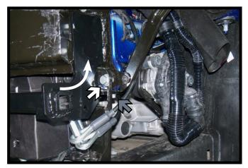
14. Slide the notched braces onto the baseplate and rotate into position on the vehicle. Start the outer existing brace bolt (white) and a 8MM-1.25 x 30MM bolt with a 8MM flat and lock washer into the underside hole of the baseplate (gray). Do this on both sides of the vehicle. Level and clamp the baseplate into position.
