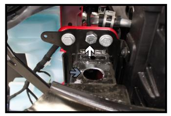
Install a 1/2"-13 x 1-1/2" bolt and 1/2"-13 whiz lock nut in the existing frame hole (white).
