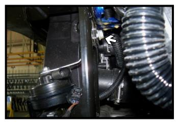
Using a T50 Torx, remove the screw from the backside of the horn bracket. Disconnect the wiring and set the horn aside. Do this on both sides of the vehicle.
