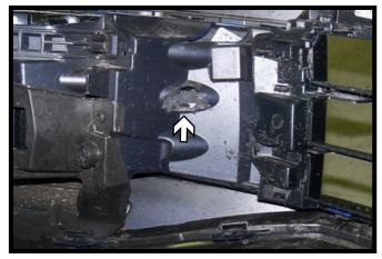
20. On the backside of the fascia, trim off material from the rib for baseplate clearance. Do this on both sides of the fascia.
