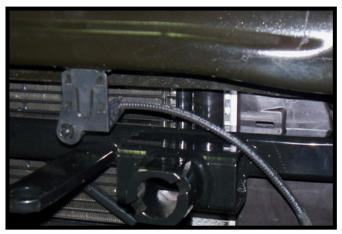
Reinstall the air temperature sensor.
