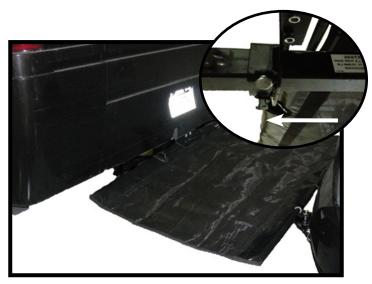
Hook up the tow bar to the towed vehicle per the tow bar instructions. Slide the front arm torwards the motorhome along the receiver mount until the screen is tight, then tighten the bolts on the underside to secure in place.
