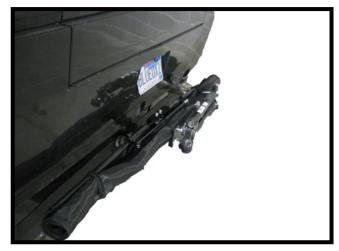
When not in use, roll the KarGard™ II up and secure with the attached velcro strips.
