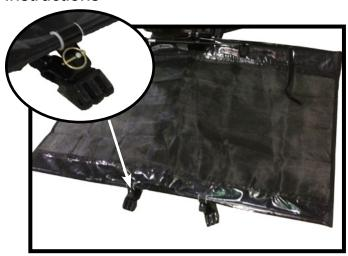
2. Slide the KarGard™ II onto the receiver tube of the tow bar, then install the tow bar onto the towing vehicle per the tow bar instructions. Extend the legs of the tow bar until the leg support lines up to the holes in the clamp brackets. Install the 3/16" linch pins to secure together.
