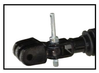
Using the 3/4" Socket and wrench, replace the existing bolts of the tow bar legs with the leg supports and 1/2"-13 essna jam nuts.
