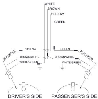
Note: Original inventory of the wiring kits were received with red/green/white wiring. The newer inventory has the standard black/brown/white wiring.
