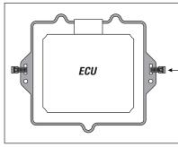
If there is no other mounting option, use at least two Large Nylon Ties to secure ECU to the location determined in Planning the Install section.
