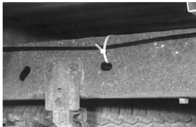
7. Cut off the air line, leaving approximately 12" of extra air line. A clean square cut will ensure against leaks. Insert the air line into the air fitting. This is a push-to-connect fitting. Simply push the air line into the 90° swivel fitting until it bottoms out (9/16" of air line should be in the fitting).
