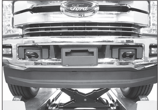
(Fig 6) Remove plastic air dam from bumper
