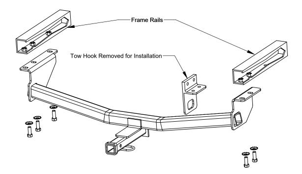
Note: Some models are equipped with appearance panels that cover the frame rails. Prior to installation remove the appearance panels. Return panels and plastic push pin fasteners to vehicle owner.
