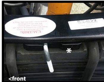
<front Place PSP-7 on top of spring plate flat side up facing, with groove toward the front
