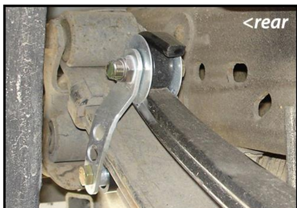
Adjustable pre-load and ride height [fnt/rear]
