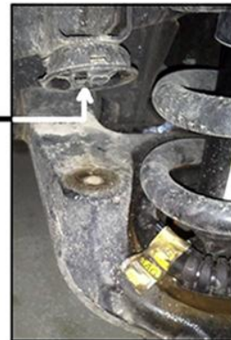
OE Bumpstop removed
