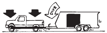
Weight distributing hitch transfers loads to frame and to both axles of tow vehicle for safer stops and smoother ride.
